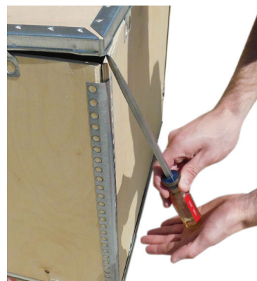
Figure 4: Removing the lid. It may help to tap the corner of the lid to break it free of the side wall tabs. Then lift-off cover.
