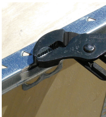
Figure 3: Flattening the tabs with pliers will allow the lid to lift off easily and it facilitates the eventual reuse of the crate.
