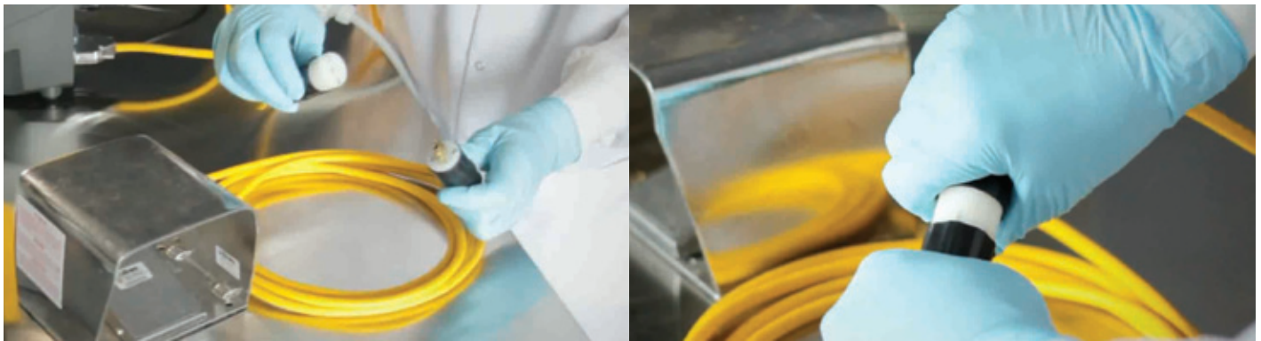
Figure 24: Locate the three pin twist lock and plug and test to secure connection.
