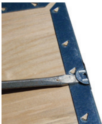
Figure 2: Unfold the cover tabs and bend them to vertical, as shown here using a flat blade screwdriver.
