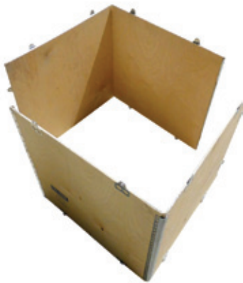
Figure 11: Two side-wall pairs after removal from base pallet.
