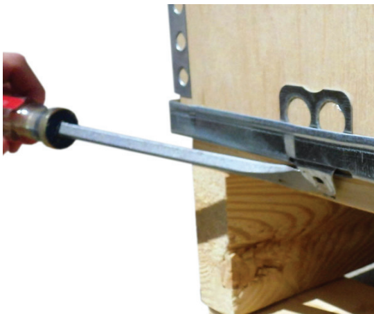
Figure 7: Note that the lower edge of the wall has two tabs. Go around the base of the crate and unfold the eight base tabs as shown here using a flat blade screwdriver.
