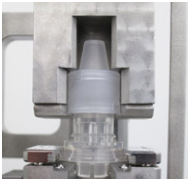
Figure 34: Fill connector in the load position, ready for fill cycle.
