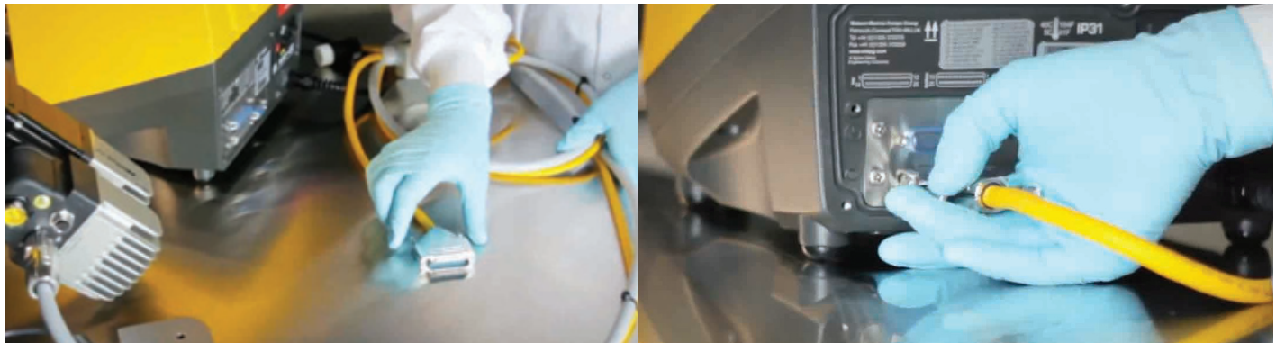
Figure 23: Locate the 25 pin connector and twist the screws to tighten the cable to pump.
