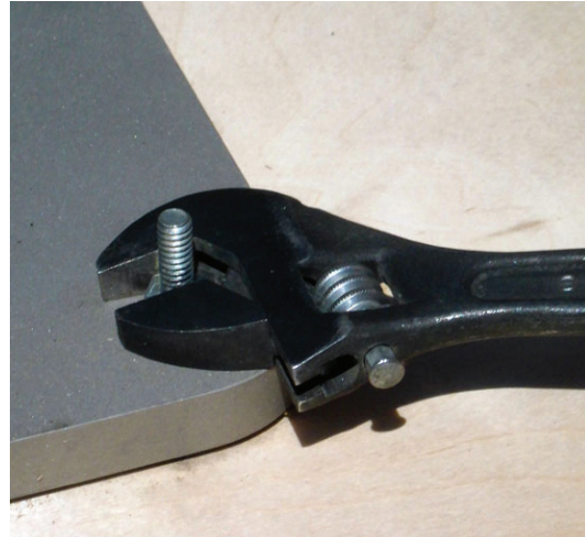
Figure 10: Unbolt base mounting hardware using a crescent wrench.
