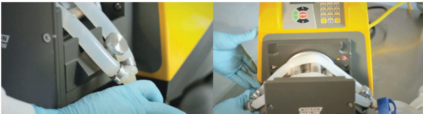
Figure 27: Install tubing over the rollers and stretch to the retention pin.
