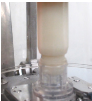
Figure 36: Nozzle fully engaged into fill stem of bag.
