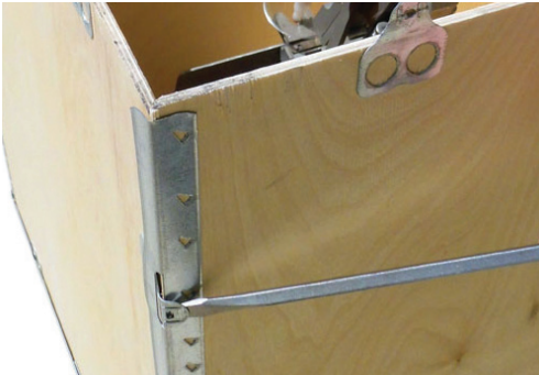
Figure 5: Unfold the vertical edge tabs. Shown here using a flat blade screwdriver.
